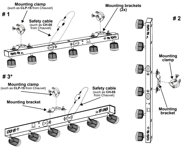
\* The 3rd mounting option is for pipe/base mounting.
